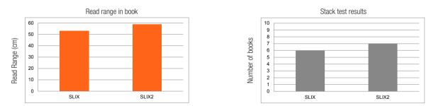
SMARTRAC TECHNOLOGY GROUP uses three different qualification methods to evaluate the quality and reliability of RFID inlay and tag products. Products are tested according to IEC 60068-2-67 (temperature and humidity), JESD22-A104-B (temperature cycling) and an in-house developed bending test. All the graphs are indicative: performance in real life applications may vary.
